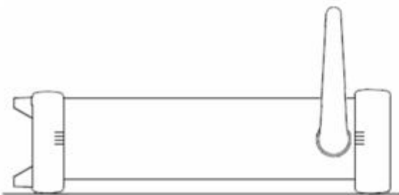
Remove handle position .(Pull to both sides until the handle is removed .)
