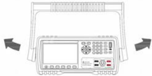
Remove handle position .(Pull to both sides until the handle is removed .)
