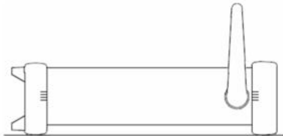
Remove handle position .(Pull to both sides until the handle is removed .)
