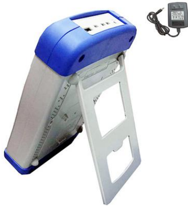
Fig 3-2 External power adapter and instrument connection
